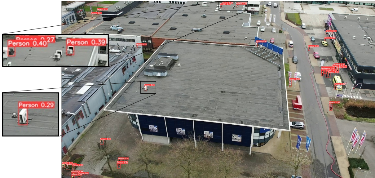
Figure 5. Example predictions of the model. Each red box is a detected human, the number stands for the prediction certainty. We zoomed in on some False Positives (rooftop objects recognised as humans).
