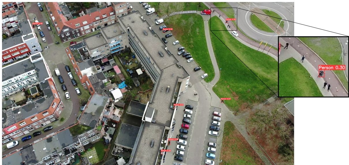
Figure 6. Example predictions of the model. Each red box is a detected human, the number stands for the prediction certainty. We zoomed in on some False Negatives (unfound humans by the model).
