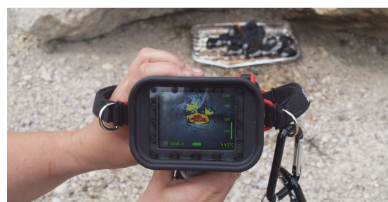
(h) Hot spot confirmed with thermal camera.
