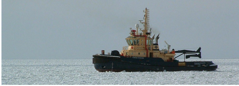
Figure 6. Tundra class coastal ice reinforced tug (Robert Allan Ltd., 2025)
