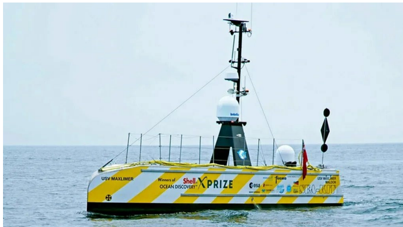
Figure 10. Fugro Sea-Kit. 12 M USV 'Maxlimer' (Amos, 2020)
