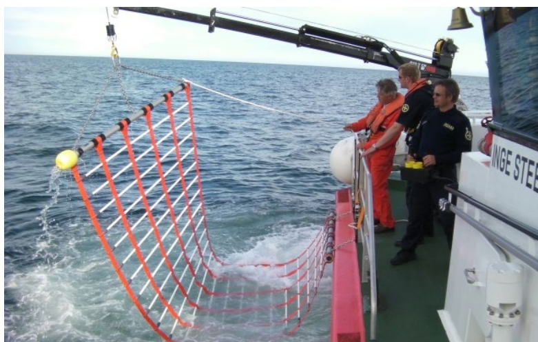
Figure 11. Dacon RSB rescue scoop on small rescue vessel, available in larger and smaller sizes to suit vessel size and configuration (Dacon, 2025)
