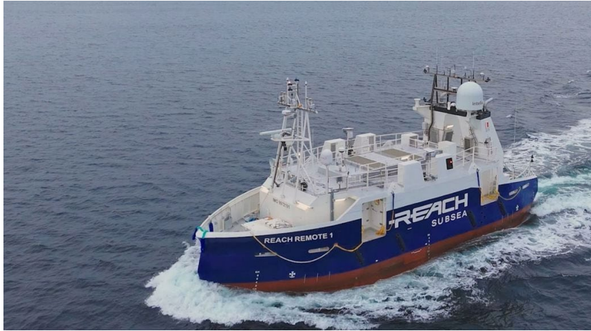
Figure 9. REACH Remote 1, 23.9 m Offshore Survey & Subsea Vessel, 2025, Kongsberg remote control / autonomous system (Kongsberg, 2025)
