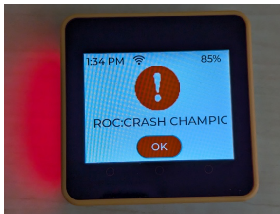
Figure 6: M5Stack Core2 's response when there is an RSS feed 911 incident
