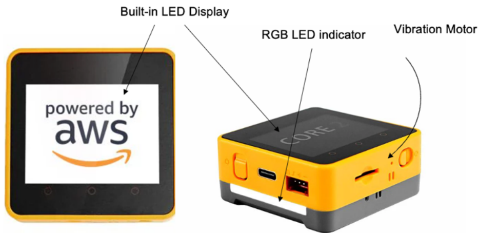
Figure 5: M5Stack Core2 Haptics and Display Screen
