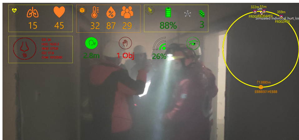
Figure 2. Example of the Modular Multi-Platform Interface (MMPI) visualization in a FR helmet HUD
