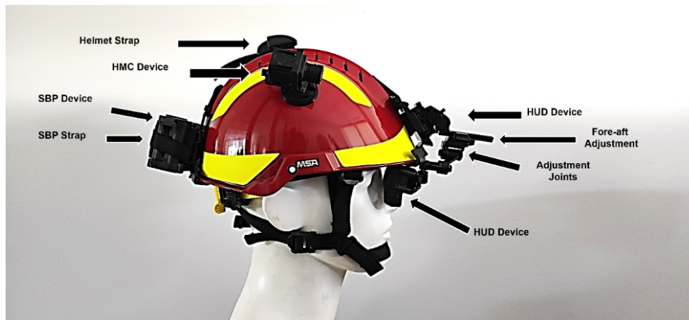
Figure 5. Draft concept of the system installed on user's helmet and the final prototype in Fernández García et al., 2023
