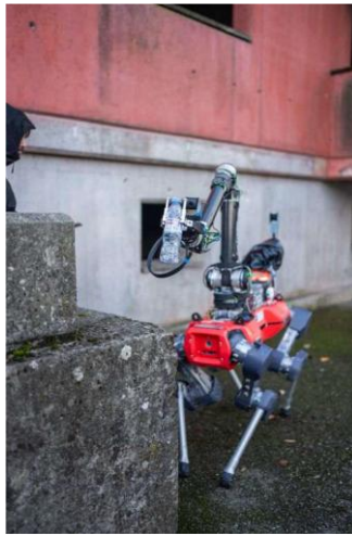
Figure 2. ANYmal with an arm performing a fetch-and-place task with a water bottle
