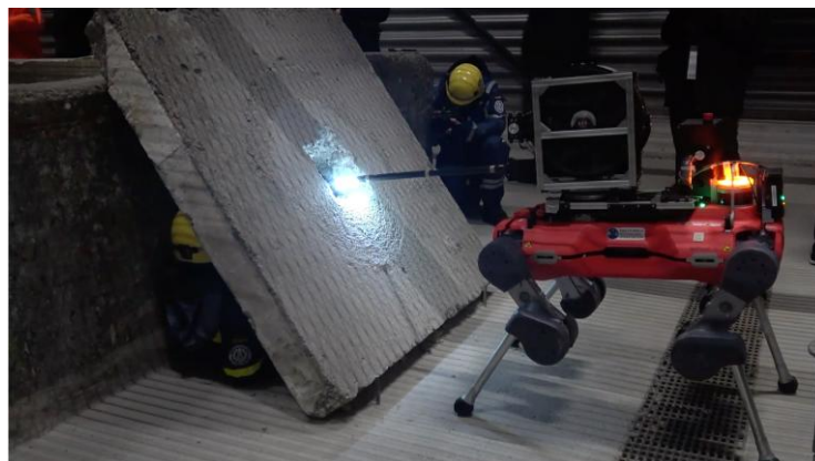
Figure 3. Search for victims through a bore hole by ANYmal and SNAKE on training site at component field test
