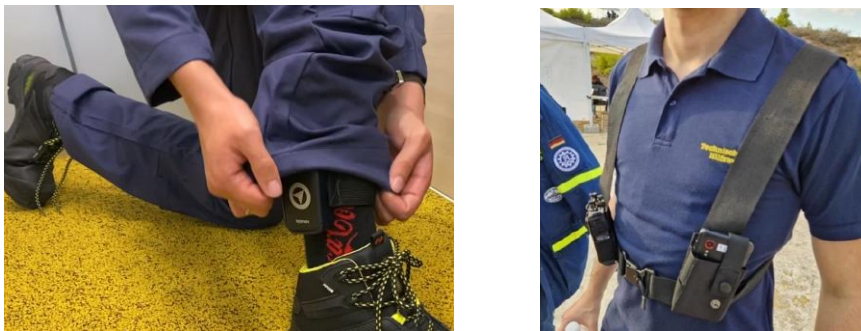
Figure 5. FR equipped with wearables for localisation (left image) and physiological monitoring (right image)
