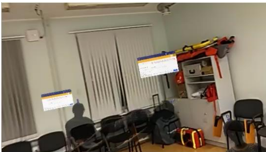
Figure 8. QR-code scan to open non-interactive 3D holograms. There are three victim holograms on the photo and above two victims head is LMS 2D hologram opened (FightARs Partners 2023)
